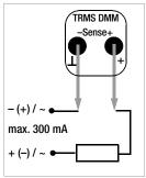
Securely connect the measuring instrument to the consuming device in series as shown (without transfer resistor).
