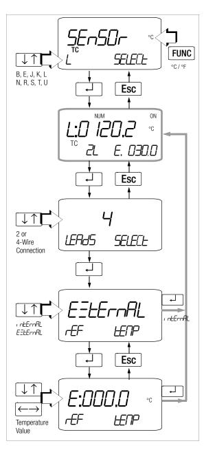
Temperature Simulation with Equalizing Lead (internal reference temperature)
