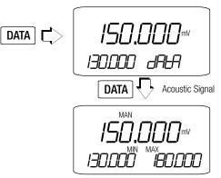
If the next stored message deviates from the first by less than 0.33% of the measuring range, two acoustic signals are generated (DATA Compare).
