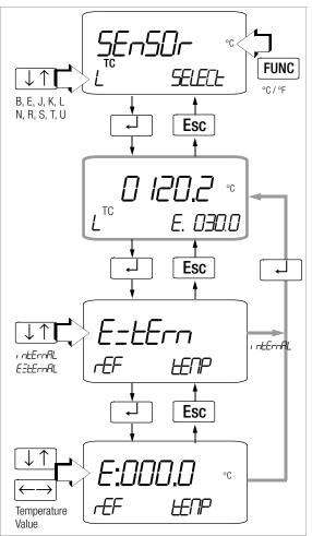
Reference temperature can be either measured with an internal reference junction, or specified with an external reference junction.
