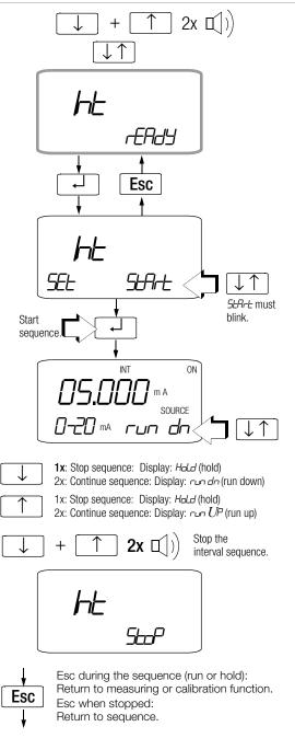
Menu Flowchart: Interval Parameters Configuration
