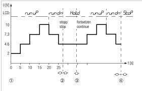
Interval parameters: Output quantity: U (0 ... 15 V range), *5LRrL* = 2 V, *End* = 10 V, number of interval steps = 3, t1 = 5 s, auto = Yes (yes for automatic sequence)
